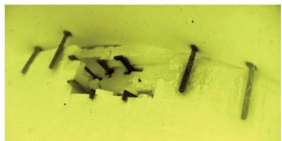
Endoscopic inspection of the gable wall with water-cooled supports.
