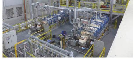
furnace must, on the contrary, provide a long residence time to allow for gas release and good refining.
