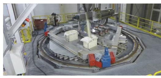
furnace installation, including necessary materials like cooling air and cooling water with their respective piping and cabling. During the engineering phase, this was supported by 3D media design.
